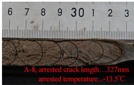
Fig.11 Fracture surface profile around crack tip
