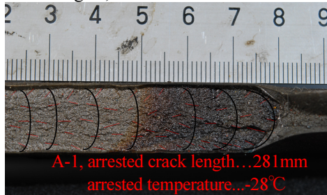
Fig.10 Fracture surface profile around crack tip
