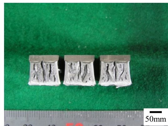
Fig. 2 Fracture surface of Charpy impact test (-140°C)
